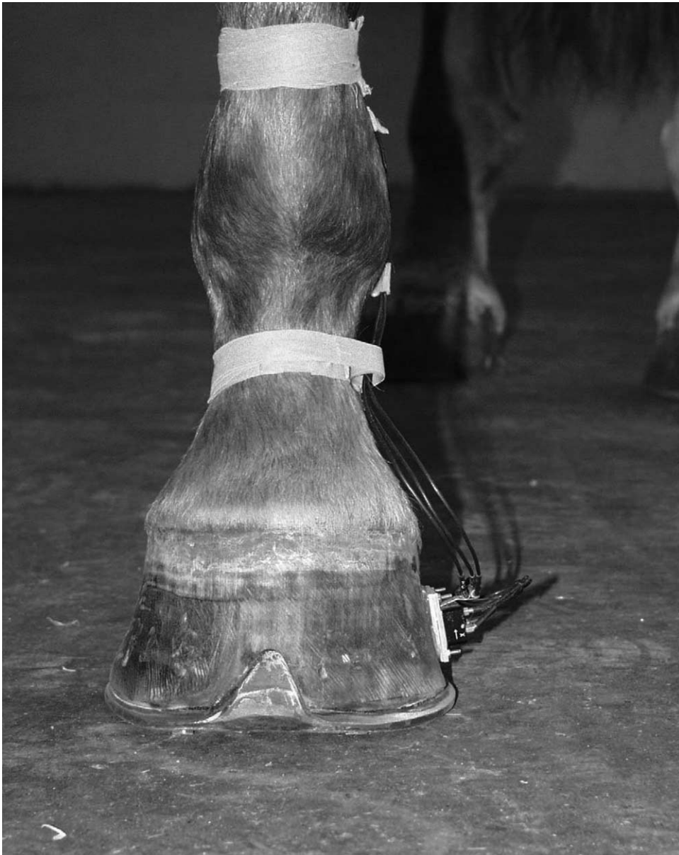
FIG. 2 Accelerations were recorded using a triaxial piezoelectric accelerometer, which was fixed to the lateral side of the left front foot
